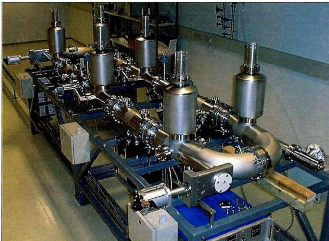
The 7 m circumference ELISA – ELeCtrostatic Ion Storage ring, Aarhus – which was commissioned this year, uses a purely electrostatic ring to store beams of charged particles – the first time this has been done since the mid-1950s.
