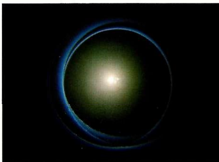
Ring the changes – first photograph of the Cherenkov radiation from a high-energy lead-ion beam at CERN.
